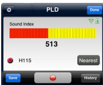
Recording using WaterPoint Pipeline Leak Detector (PLD)
