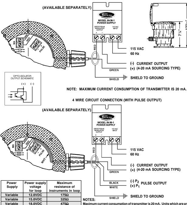
Maximum current consumption of transmitter is 20 mA. Units which are provided with only 2 output wires may be rewired for 150 ppm pulse output by stripping back the insulation on both ends of the output cables and wiring as shown above.
