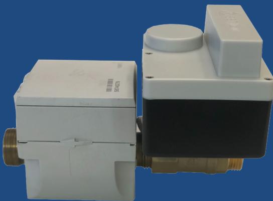
The meter neutral SET 100C Remote Smart can be retrofitted to existing meters or installed with new meters. For example, when coupled with the 5" Diehl Hydrus Ultrasonic Meter, the lay length equals the 7.5" standard meter box lay length.
